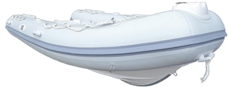
Designed to deliver the perfect balance of functionality and performance, HSF is impressive both at rest and on the move. The pronounced bow-sheer, deep V keel, large tube diameter and full-length lifting strakes of this series guarantees a great sea-going vessel and a smooth dry ride. Its stability at rest, its spacious cockpit and its heavy duty grab handles, makes the ideal platform as a dive boat, rescue/response boat or coach/support boat.
